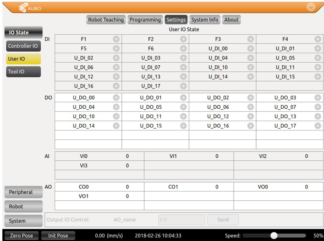
The screenshot shows the AUBO software interface with the 'Settings' tab selected. The 'User IO State' section is active, displaying a grid of digital input (DI) and digital output (DO) channels. The 'User IO' button is highlighted in yellow.
