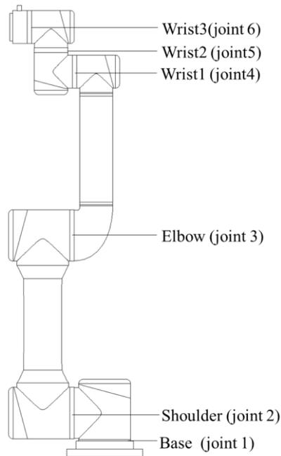
Figure 5-2 -1 Manipulator Joints
