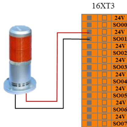
Figure 8-17 Figure robot moving output connection
