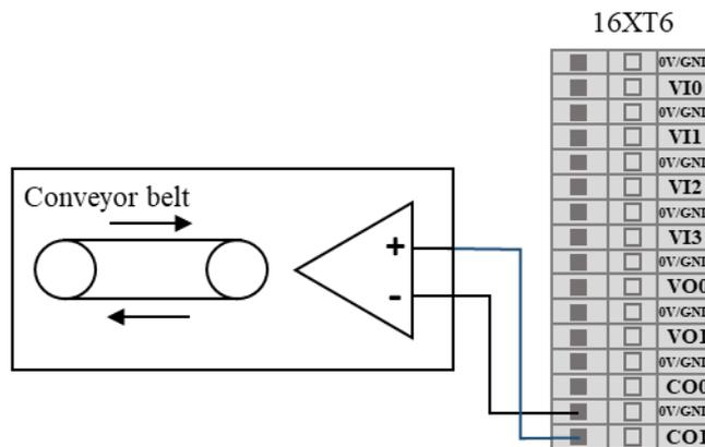
Figure 8-31 Analog current output connect to current source
