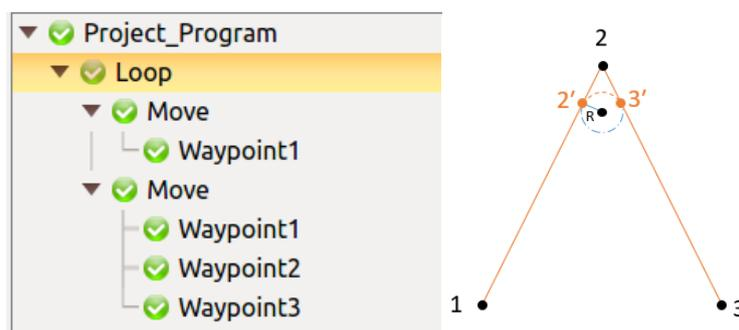
Figure 11-20 blending radius motion track
