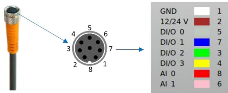
Figure 8-36 Robot Tool I/O wiring order
