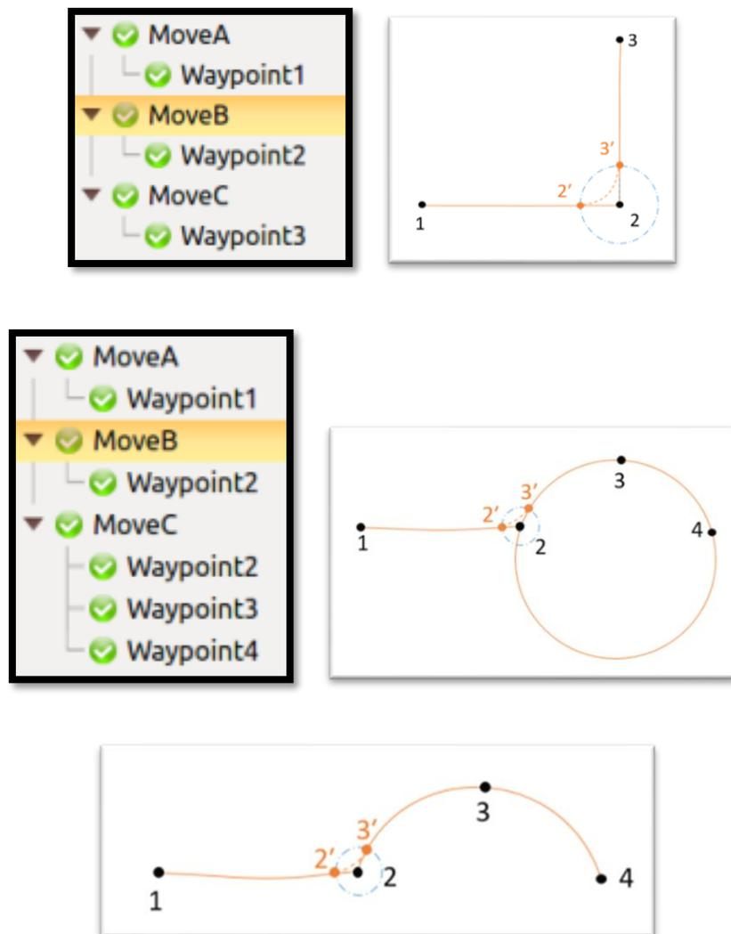
Figure 11-23 Arrival Ahead – Blend Radius Trajectory Example (Move Line and Move Track)
