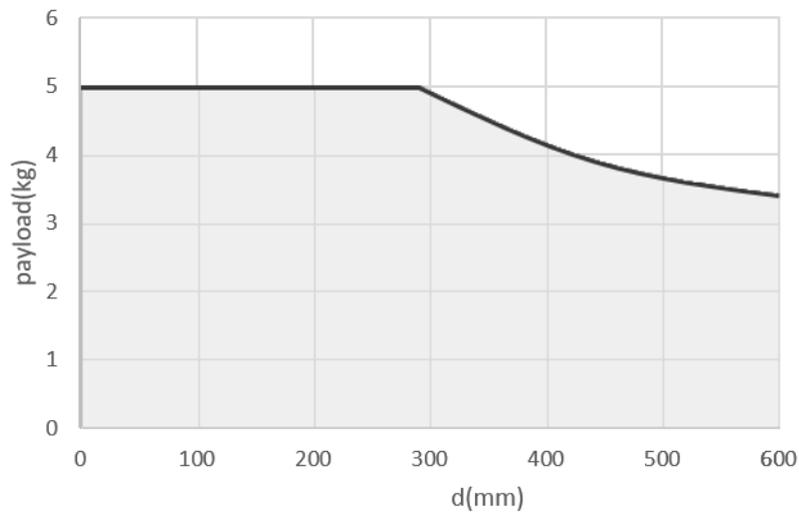
Payload of wrist has shown above, in which d-axis represent the center of gravity offset which is the distance between end-effector flange focus and tool focus.
