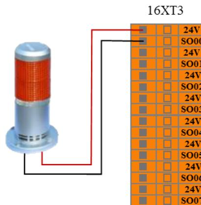
Figure 8-16 robot emergency stop output connection
