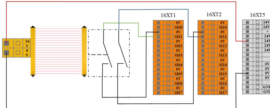
Figure 8-6 Safeguard stop input (Internal Power Supply)
