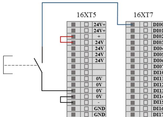
Figure 8-25 DI terminal connection button switch schematic
