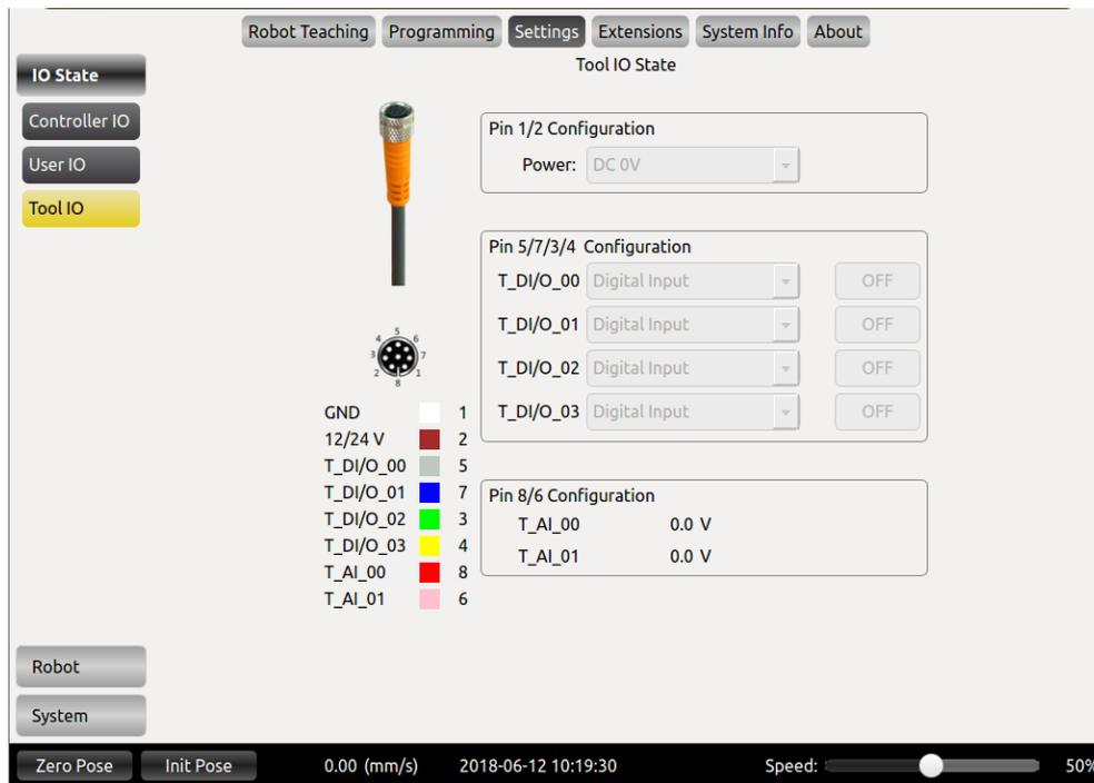
Figure 10-26 Tool I/O panel
