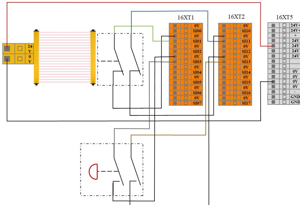
Figure 8-7 Safeguard stop input (Internal Power Supply)
