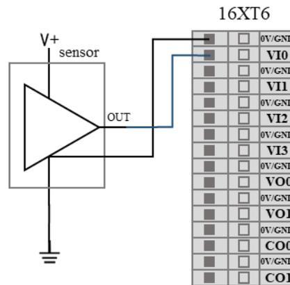
Figure 8-30 Analog voltage input connect to sensor
