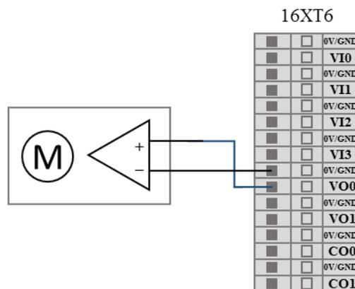
Figure 8-29 Analog voltage output connect drive device
