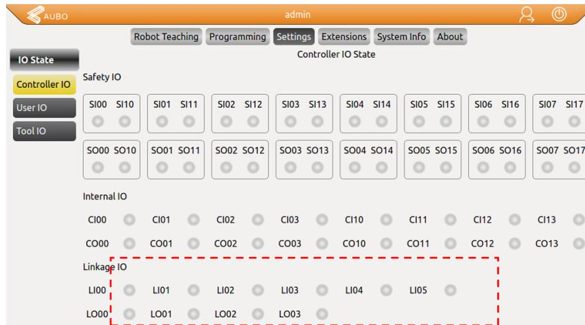
Figure 7-9 AUBOPE software "Settings" tag, Linkage IO status
