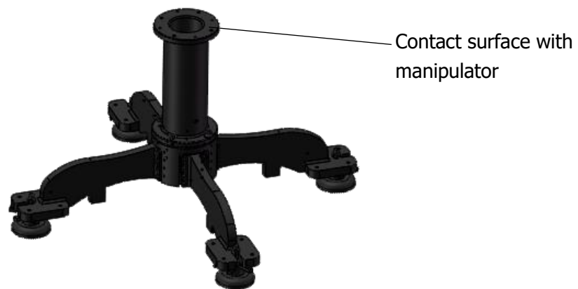
Figure 6-3 Diagram of manipulator base structure
